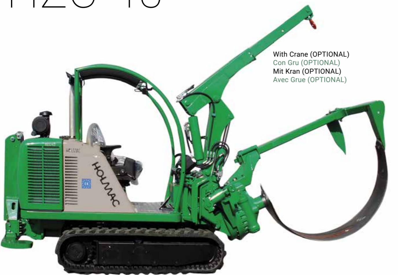
**EN** The HZC 45 represents the first step of a new range of treediggers. It's built with really new technical and mechanical characteristics to grant the best work capacity with the biggest security and results. The HZC 45 has been developed to increase the drive comfort for the operator reducing highly the vibrations and permitting a better visibility during tree-digging; besides the opening/forwarding system of the tracks allows to lift up trees with rootballs till 150 cm of diameter.
