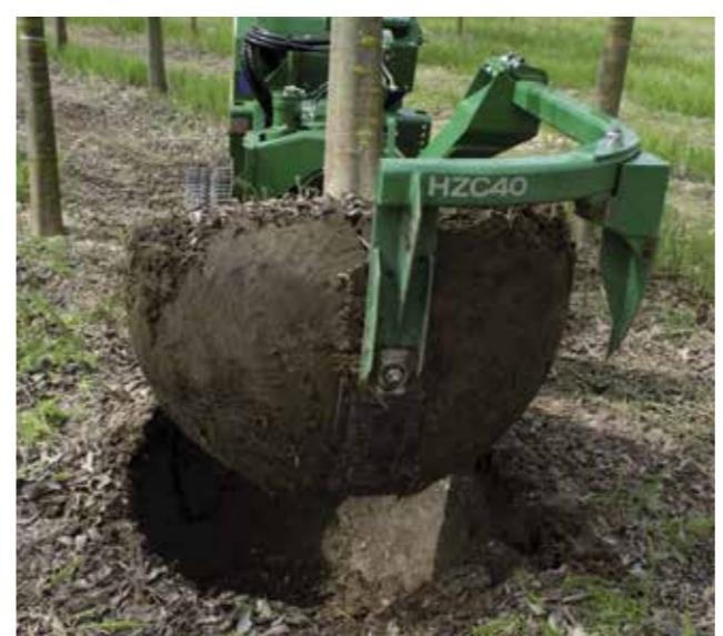
**EN** With the Treedigger HZC 40 you can dig out trees with rootballs from 40 cm to 140 cm of diameter. With the vertical lifting system you can lift the tree with its rootball out of the soil completely holding the tree in the vertical position. Comparing to the previous HZC 38, we are giving more attention to the worker, insulating totally the driver seat.
