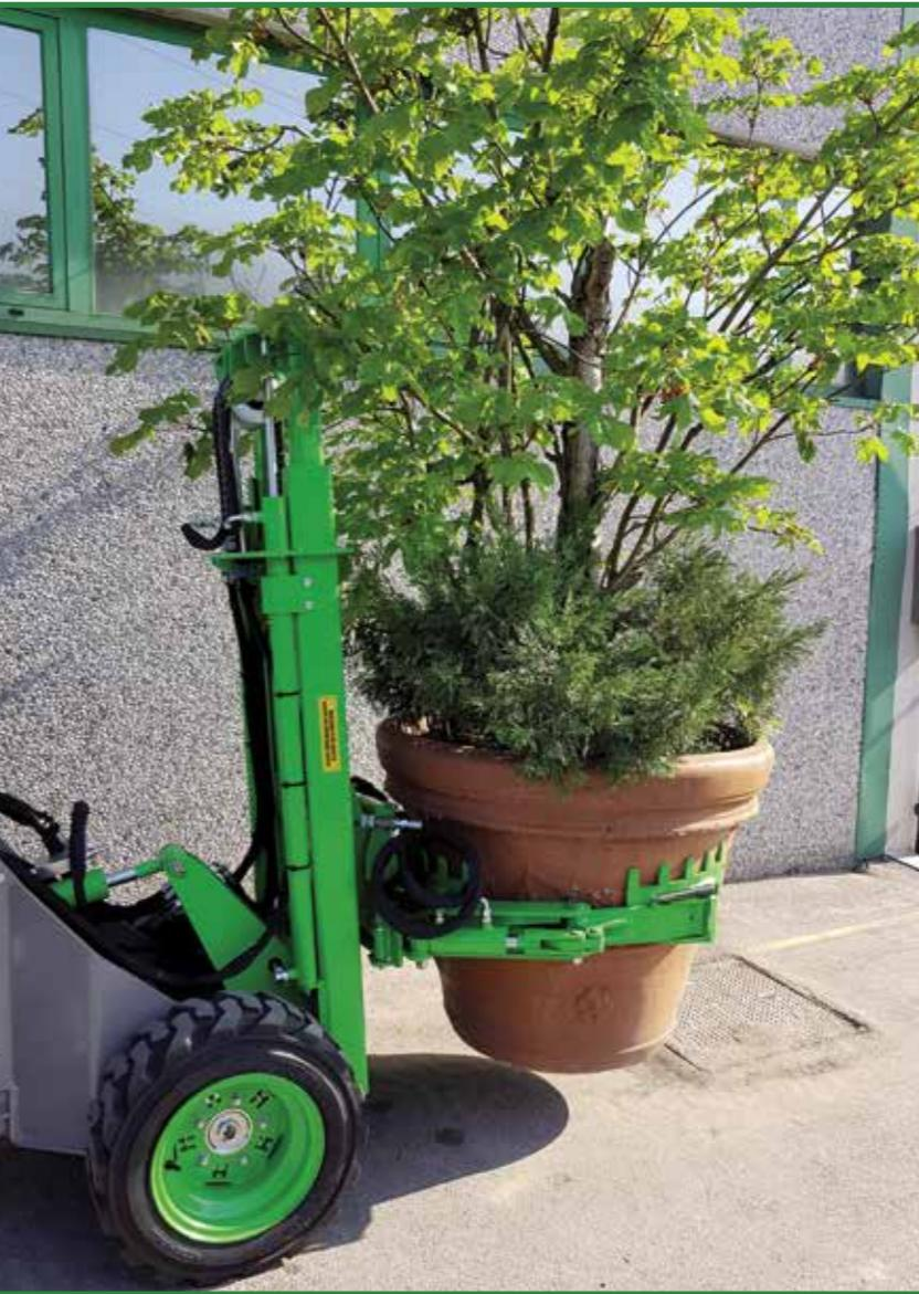
Clamp with vertical lifting system
