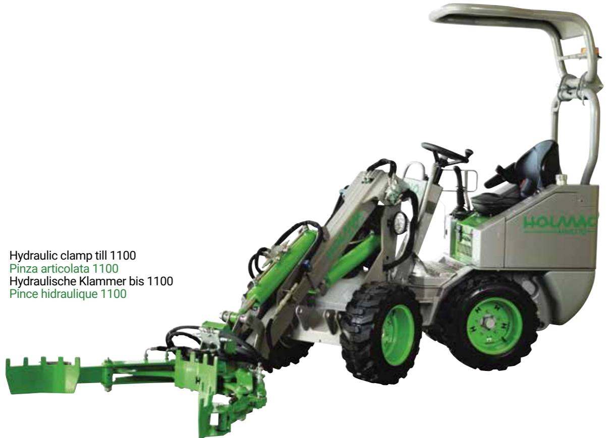
**EN** The HMU 70 Telescopic is an extremely compact and indispensable machine for nurseries. Thanks to the quick release it is possible to mount a series of accessories designed for the nursery. The telescopic arm facilitates loading and unloading, handling of potted plants, pallets and other materials. The four-wheel drive and the central joint guarantee better stability on all types of soil.
