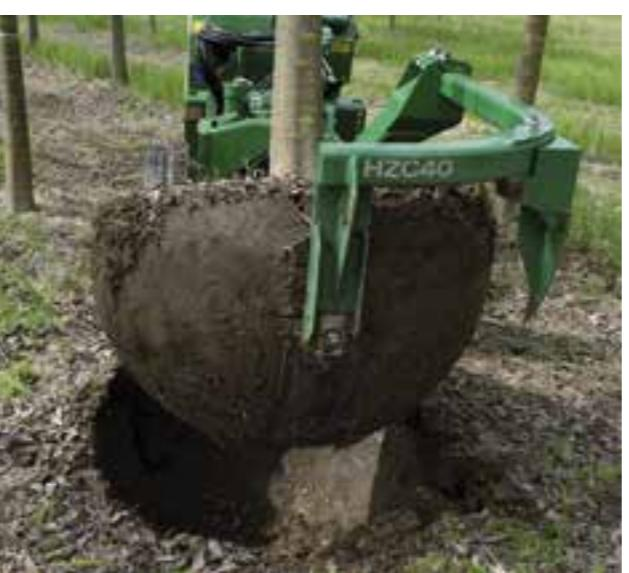
**EN** With the Treedigger HZC 40 you can dig out trees with rootballs from 40 cm to 140 cm of diameter. With the vertical lifting system you can lift the tree with its rootball out of the soil completely holding the tree in the vertical position. Comparing to the previous HZC 38, we are giving more attention to the worker, insulating totally the driver seat.
