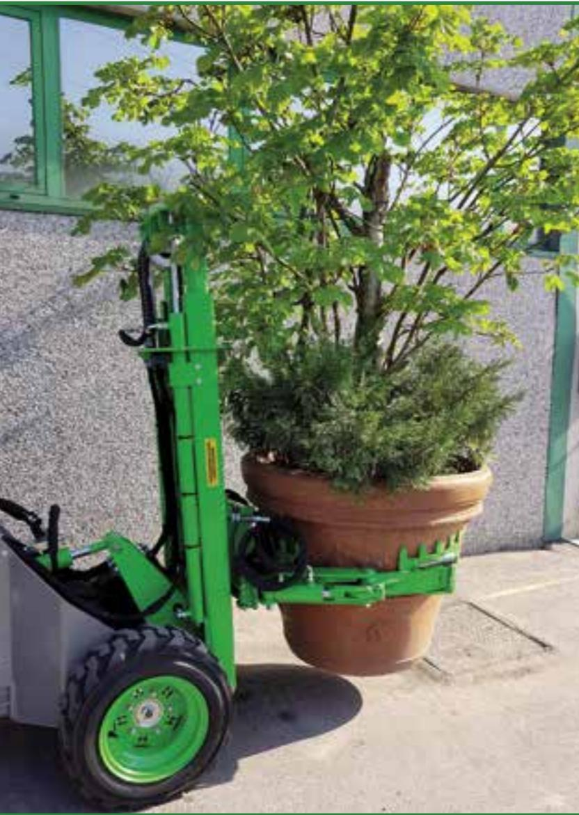
Clamp with vertical lifting system
