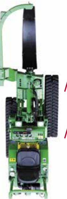
**EN** With the Treedigger HZC 40 you can dig out trees with rootballs from 40 cm to 140 cm of diameter. With the vertical lifting system you can lift the tree with its rootball out of the soil completely holding the tree in the vertical position. Comparing to the previous HZC 38, we are giving more attention to the worker, insulating totally the driverseat.
