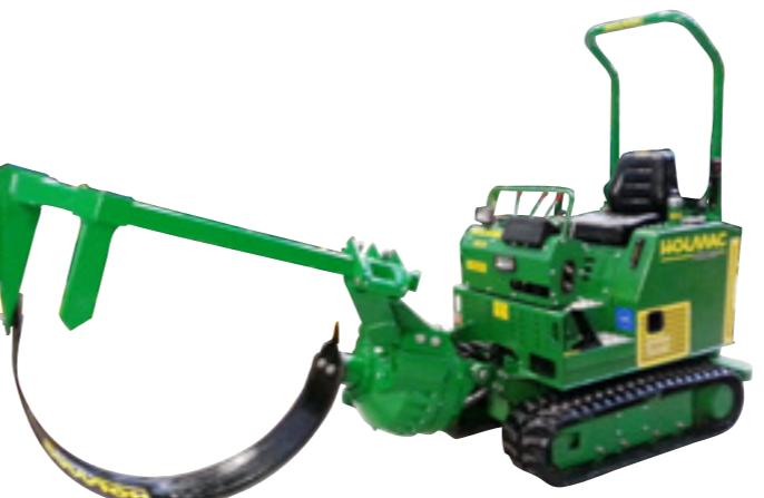
**EN** With the Treedigger HZC 38 you can dig out trees with rootballs from 40 cm to 140 cm of diameter. With the vertical lifting system you can lift the tree with its rootball out of the soil completely holding the tree in the vertical position. Comparing to the previous HZC 37, we are giving more attention to the worker, insulating totally the driver seat.
